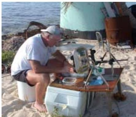
*Darryl L. Felder at CBC using his custom-made photographing machine which consists of a modified Igloo cooler and some odd items including pick-up truck side rear-view mirrors. (Photo by Rafael Lemaitre)*
